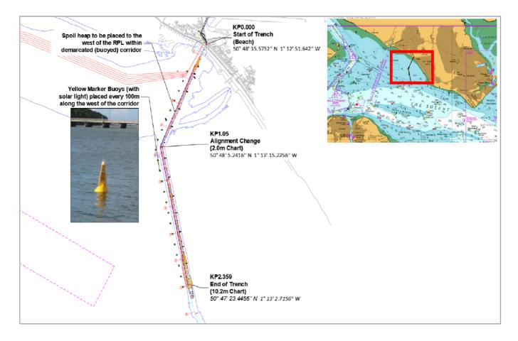
2. The 2.3km works corridor will be demarcated along the west of the trench (60m to the west) by lit Yellow Marker Buoys (FI Y 5s) located every 100m.
