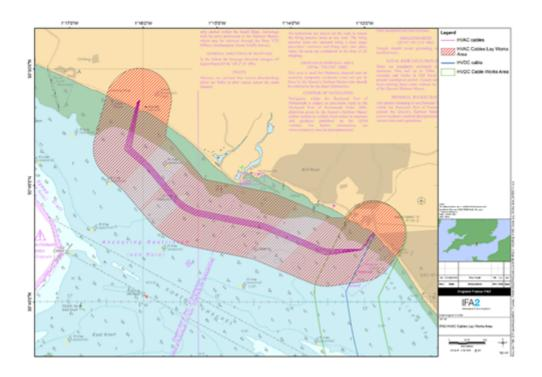
3. NP289 will manoeuvre along the cable route using a combination of anchors and spud legs, which will be deployed within the areas shown at the diagram above. Vessels should coordinate with local safety support and guard vessels for any clarifications on the mooring lines and anchor positions; anchors will be marked with buoys. Vessels should always pass a safe distance around the operations and never between the vessel and an anchor in use, where mooring cables under tension will be present.
