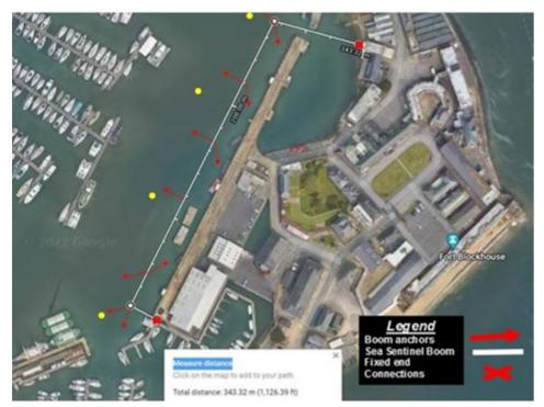
2. The boom will be attached to the shore at either end of the jetty structure and anchored to the seabed so that the boom sits approximately 15 metres off the jetty face.
