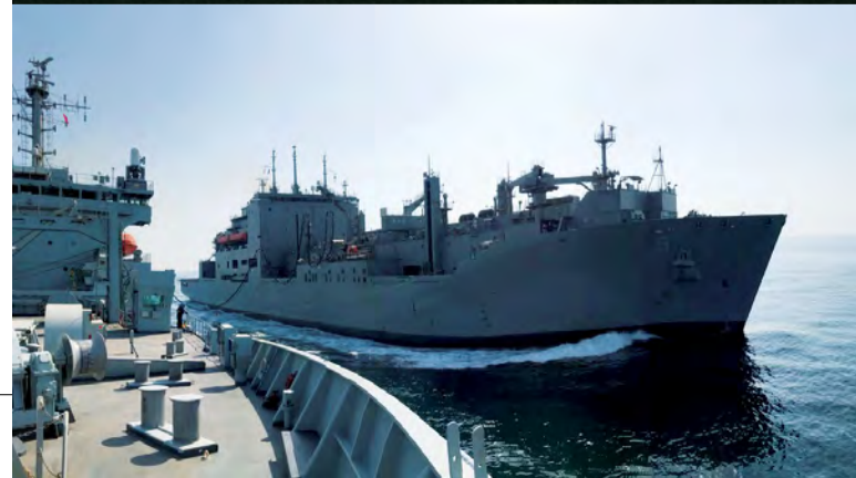
● Below, RFA Fort Rosalie carries out a RAS with the USNS Matthew Perry
