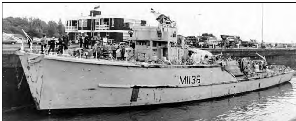
● The raised wreck of HMS Fittleton shows the extent of the damage she sustained when she was struck by HMS Mermaid, capsized and subsequently sank
