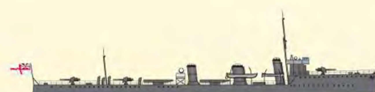
16 'K CLASS' (++++) Displacement: 984 tonnes Armament: 3 x 4" Length: 81.5 m Beam: 8.1 m torpedo tubes Speed: 32 knots Complement: 77
