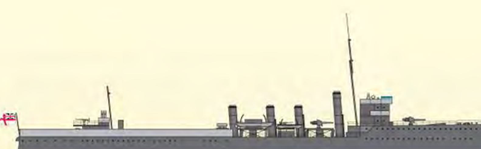
ABDJEL Displacement: 1,700 tonnes Armament: 2 x 4" Length: 99 m Beam: 9.7 m 66 mines Speed: 34 knots Complement: 104
