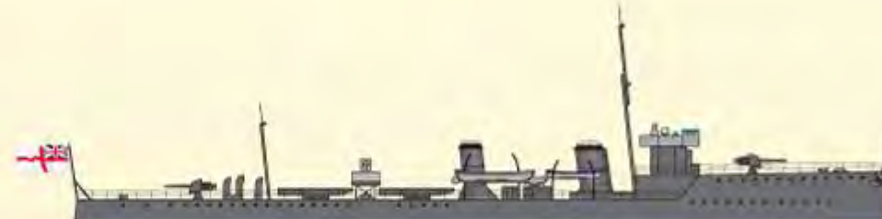
9 'I CLASS' Displacement: 790 tonnes Armament: 2 x 4", 2 x 3" Length: 76.8 m Beam: 8.1 m torpedo tubes Speed: 35 knots Complement: 77
