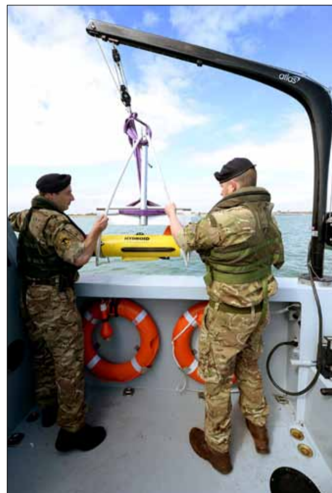
● CPO 'Fingers' Dumbleton (left) and a MASTT shipmate prepare to put a Remus 100 in the Solent on a test run and (below) a Remus scan of a wartime LST sunk in Lyme Bay during D-Day rehearsals in 1944
