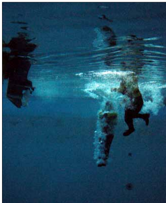
● Lifejackets are tested in jumps from the 4m platform at the RNLI training facility in Poole
