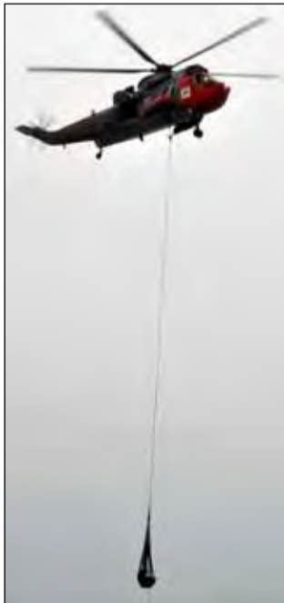
● A Sea King from 771 Naval Air Squadron with the calf as an underslung load
