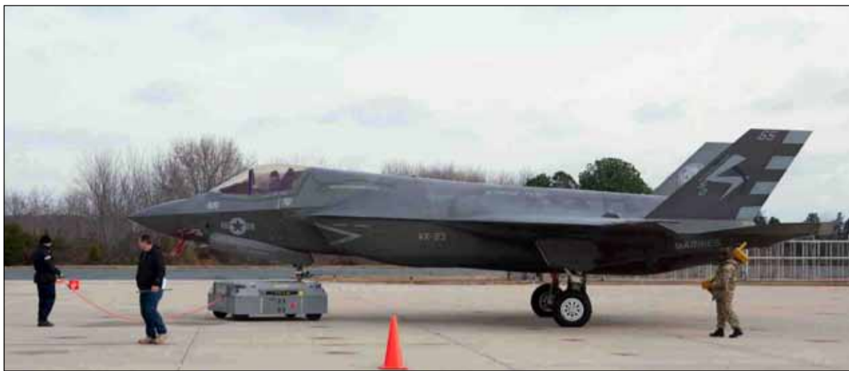
● PO Paul 'Knocker' White visited the US Naval Air Station Pax River in Maryland to get to grips with the new aircraft handling kit which will be used to move the F35s around on the Queen Elizabeth-class aircraft carriers
