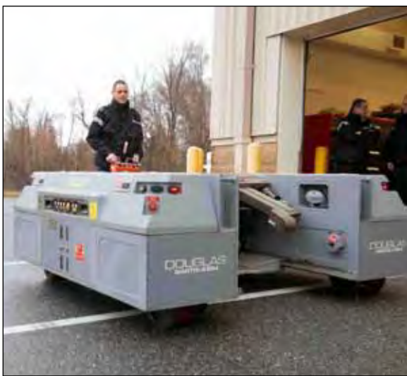
● PO Paul 'Knocker' White visited the US Naval Air Station Pax River in Maryland to get to grips with the new aircraft handling kit which will be used to move the F35s around on the Queen Elizabeth-class aircraft carriers
