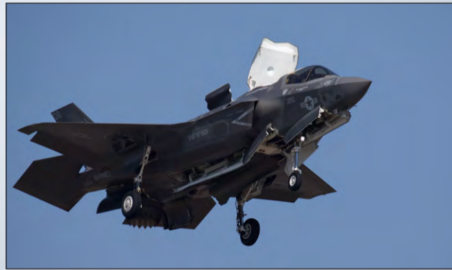
● A UK pilot in an American F-35B perfects his vertical landing skills over the hover pad
