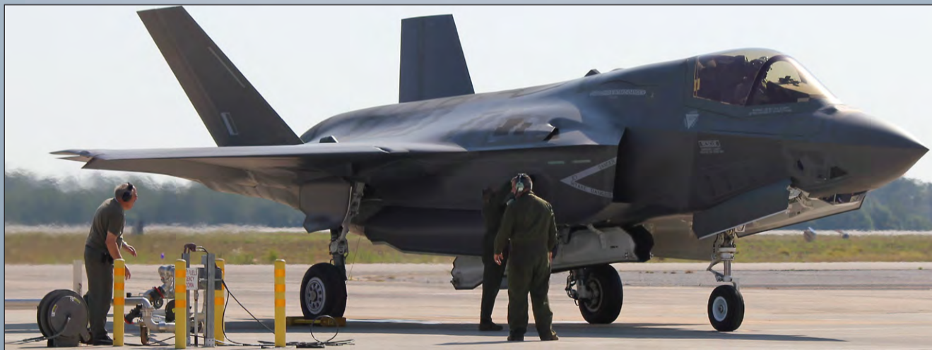
● Engineers carry out a hot-pit refuel of BK-2 at Eglin Air Force Base
