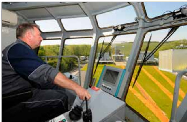
● A container begins its 40-second journey from the HRAS rig across 55 metres of 'sea' to the mock up of the reception area on HMS Queen Elizabeth – as directed by Rolls-Royce's John Trehwhitt at the console of the RASCO high up above the site (left)
