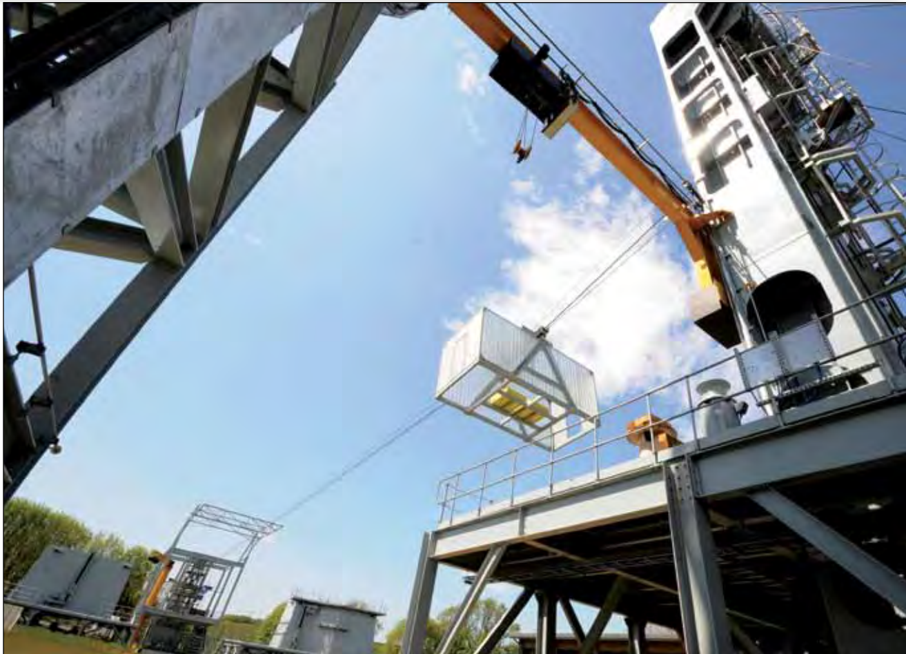
● A container begins its 40-second journey from the HRAS rig across 55 metres of 'sea' to the mock up of the reception area on HMS Queen Elizabeth – as directed by Rolls-Royce's John Trehwhitt at the console of the RASCO high up above the site (left)
