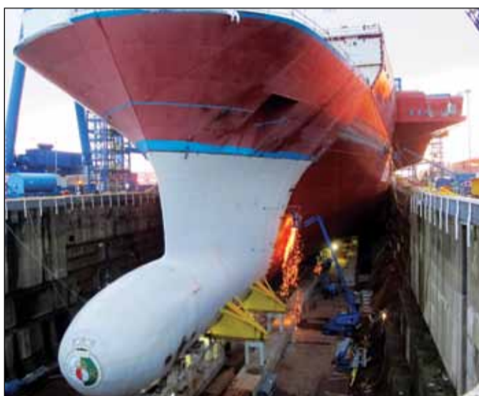
● Island hopping... (Top) Tugs shepherd the barge carrying the forward island out of Portsmouth Harbour and (above) out into the Solent as the hovercraft scurries across to the Isle of Wight while (below) a welder works on the lower bow section shortly after the middle bow was craned into place by Goliath
