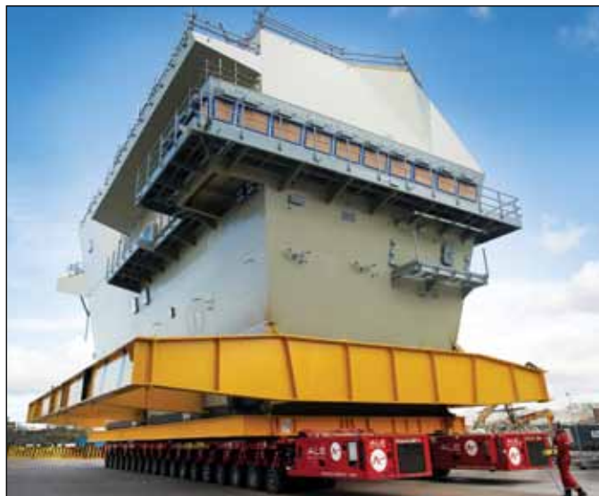
● The aft island – Upper Block 14 – of Queen Elizabeth is rolled out of Scotstoun on the Clyde last month Pictures: Aircraft Carrier Alliance
