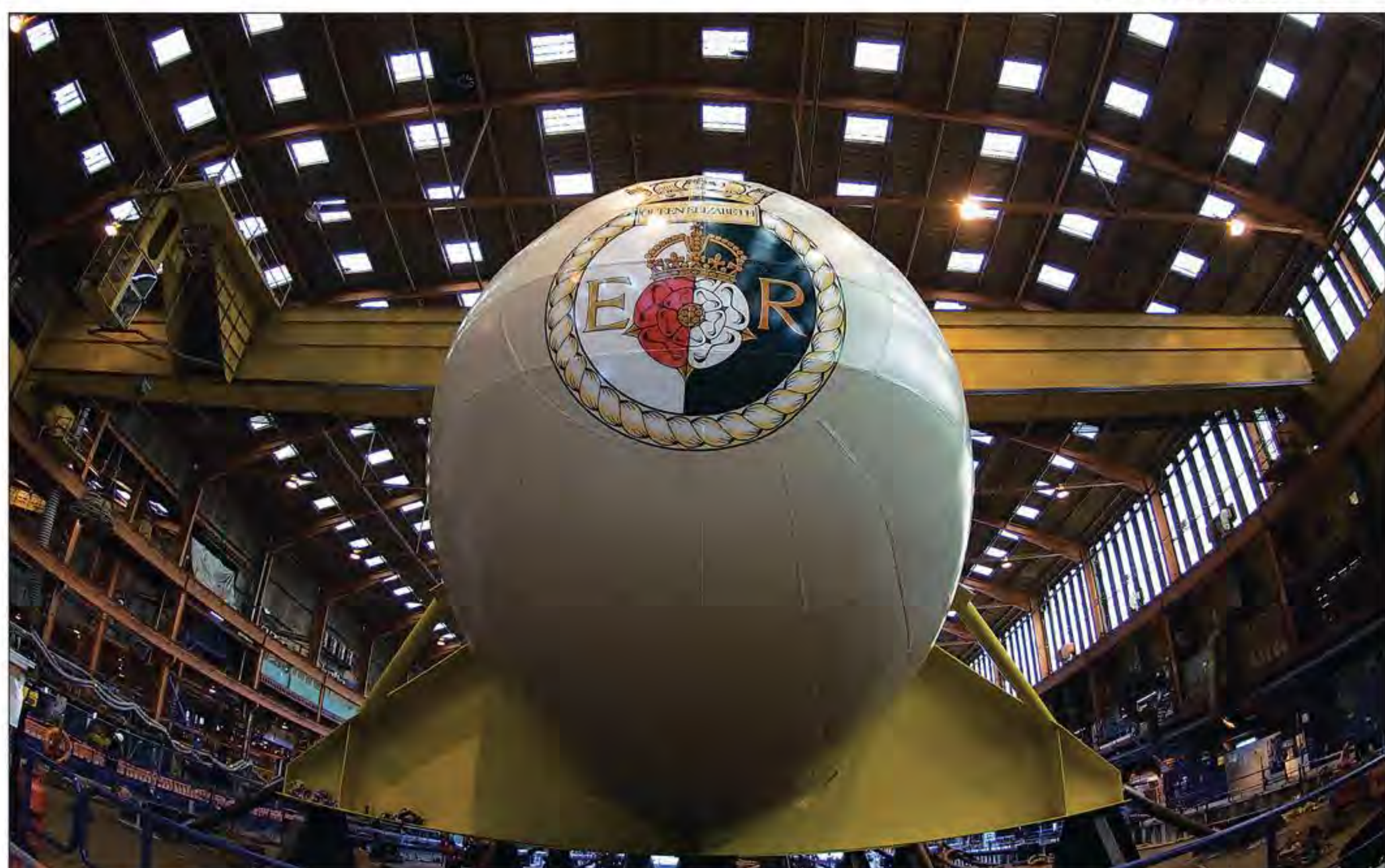
● The bulbous bow of HMS Queen Elizabeth in the Main Building Hall at Babcock's Appledore shipyard
