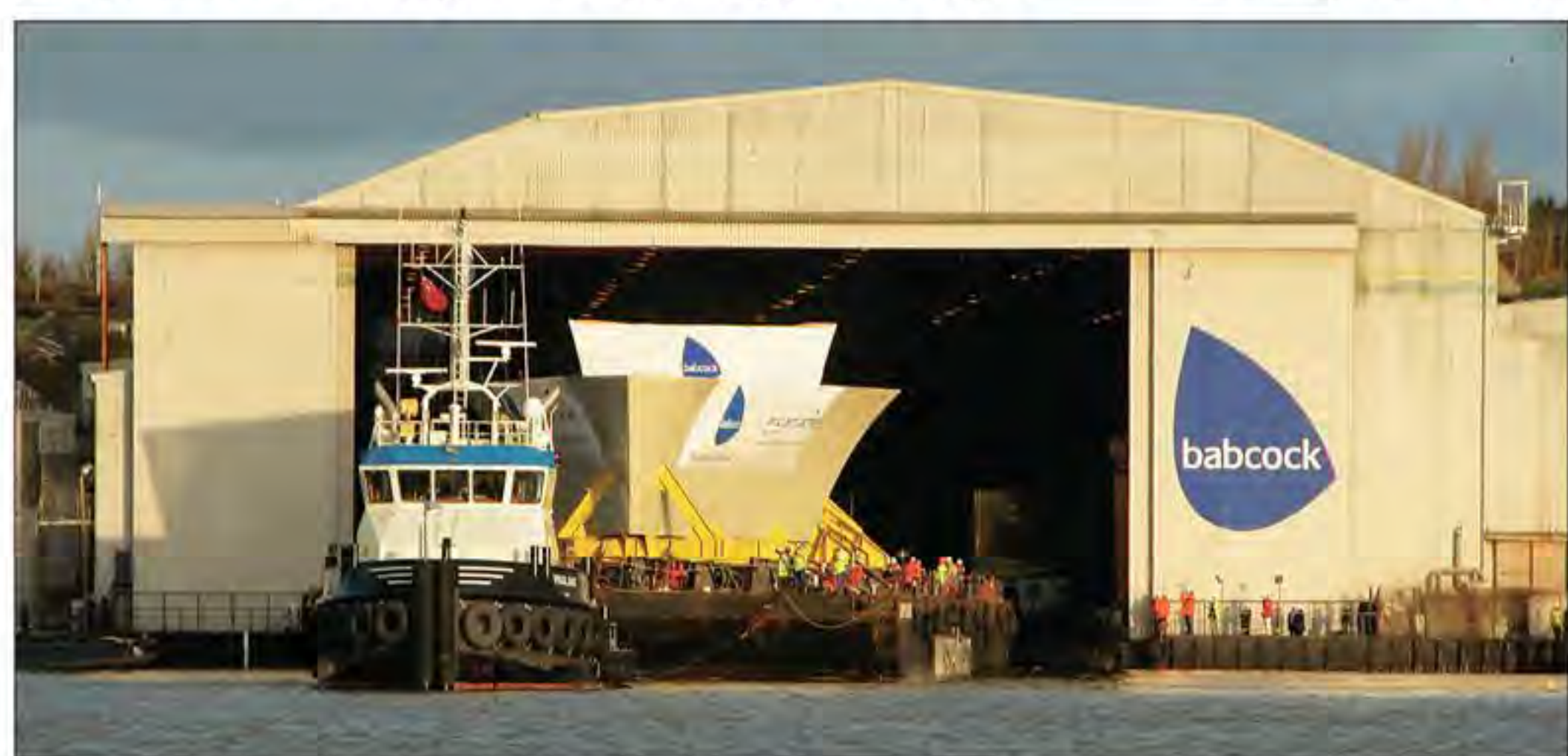
● The bow sections are towed from the shed at Appledore by the tug Vigilant
