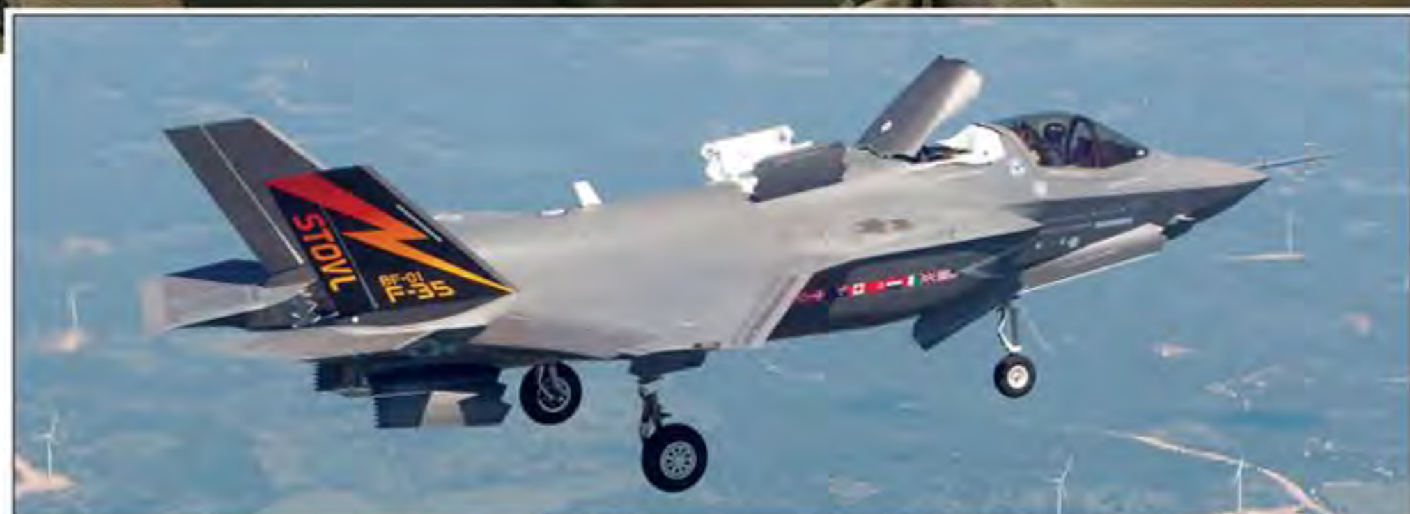
● Lightning II, seen above in 'converted' flight mode with STOVL doors deployed
