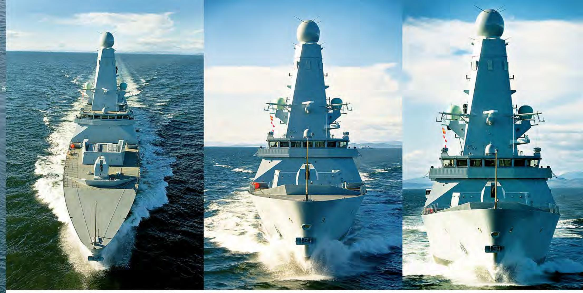
There are few 'bumps' on Daring's upper deck, no boats, capstans, lockers sticking out. The lines of the hull are as flush as they can be.
