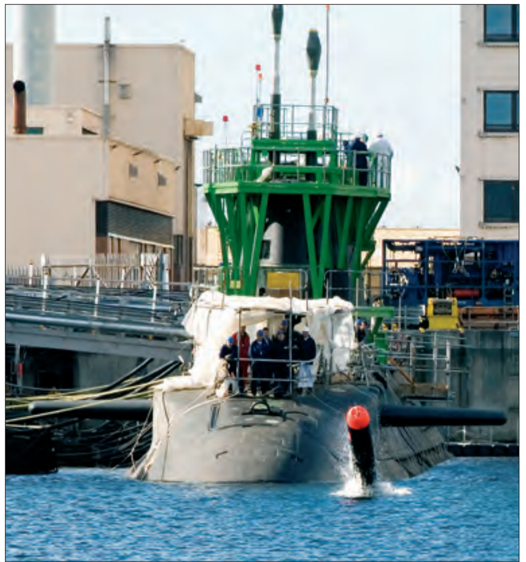
● Engineers watch as a dummy Spearfish torpedo shoots into Astute's basin
