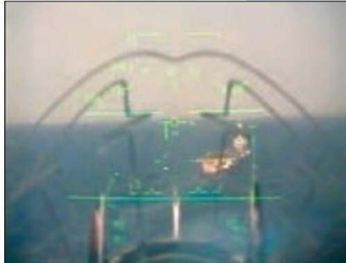
● HUD for heights... A cockpit-eye view of the approach to the Charles de Gaulle from the VAAC Harrier and (right) a sizeable number of French sailors watch as the specially-adapted jump jet prepares to land on France's flagship
