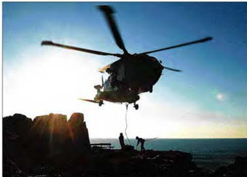
● A Merlin helicopter from RNAS Culdrose lifts gravel to help restore a coastal path
