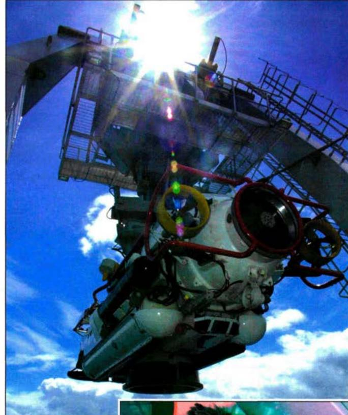
(Above) British submersible LR5 is hoisted back on board Swedish navy submarine rescue ship Belos after successfully linking with Swedish submarine Gotland almost 400ft deep in the Sound of Raasay, Western Scotland.
