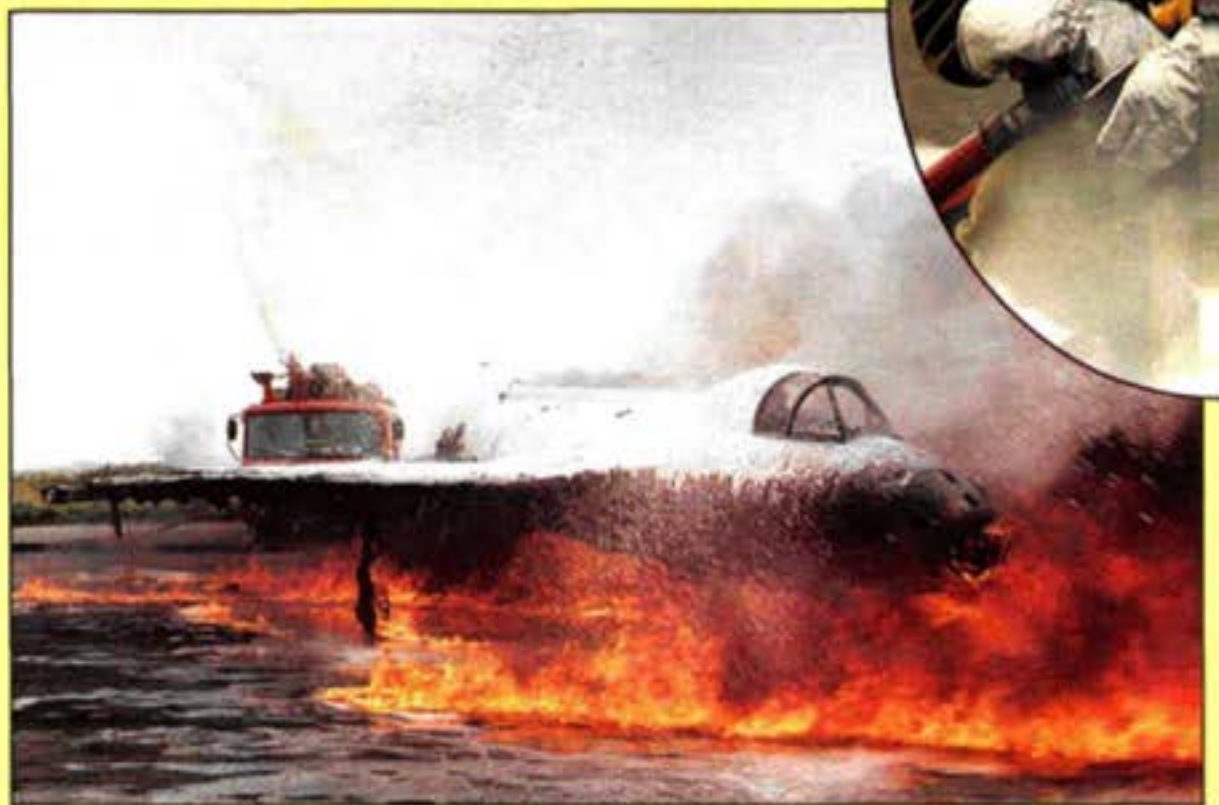
A Mark 10 crash rescue vehicle at Predannack Airfield smothers a blazing aircraft with foam
