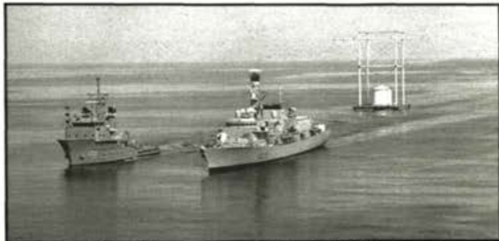
● Above: USNS Mohawk, left, tows the Empress II as it bombards HMS Lancaster with magnetic waves
