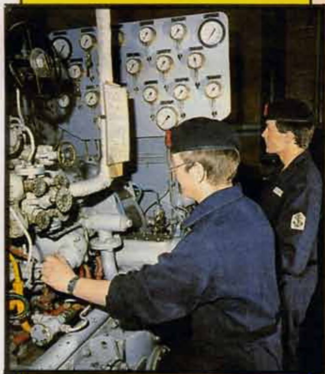
Looks as complicated as all those dials in the cockpit of an airliner, but A/LMEA Polly Pollard and A/LMEA Mac Lisle are quite at home working through the pre-start checks on a turbine alternator fitted to Y100, Y136 and Y160 Leander class frigates. It forms part of their training at Caledonia.
