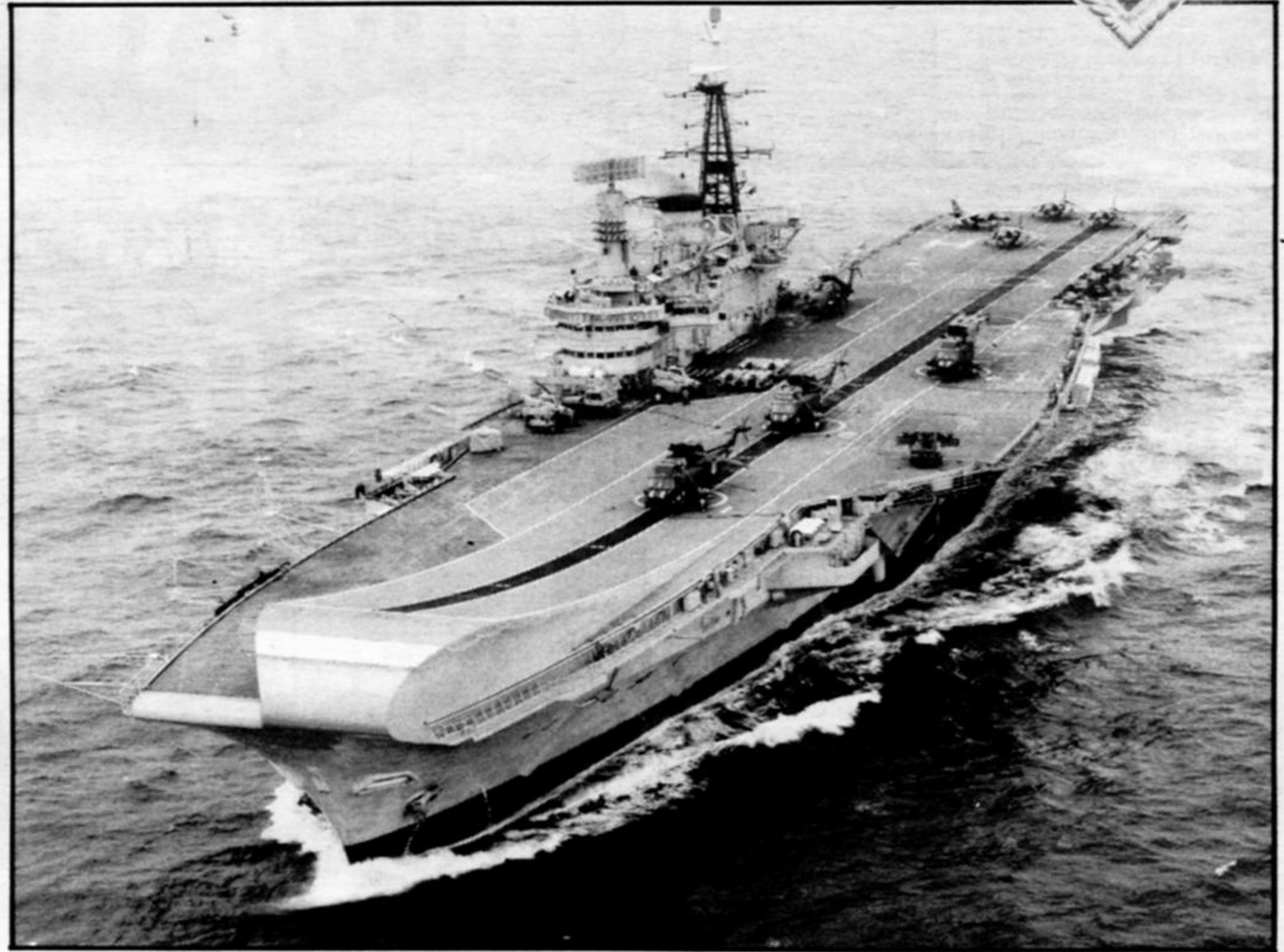
H.M.S. Hermes conducting trials after her "nose job" refit. Sea Harriers, Sea Kings and a Wessex helicopter can be seen on her flight deck, drastically remodelled for and to provide the 22-year-old carrier with a "ski-jump" take-off ramp.
