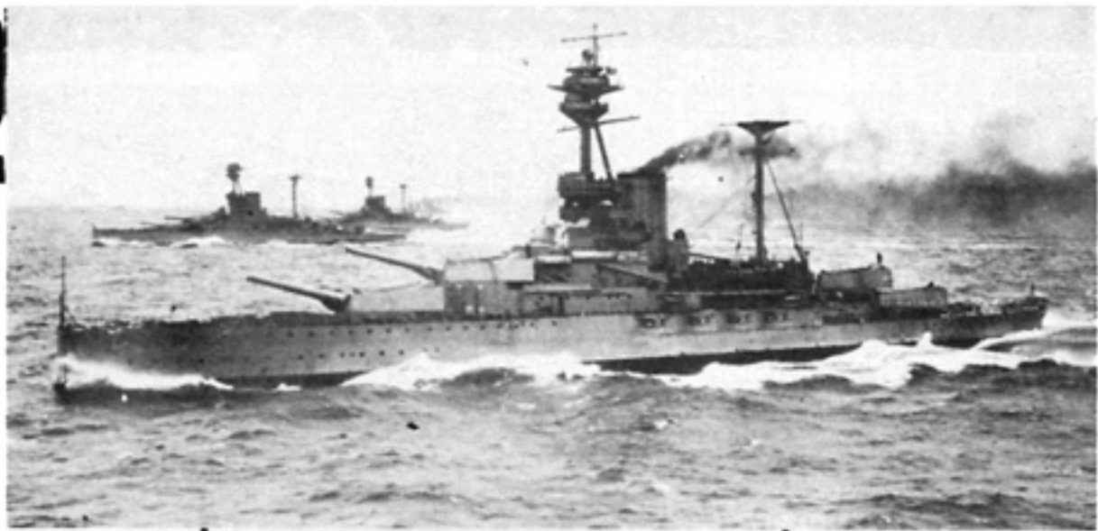
H.M.S. Royal Sovereign on exercises with the Grand Fleet in 1916, showing a searchlight on the fore-top roof, and the training scale on "Y" turret. The two ships of the Royal Sovereign class in the background each show a different arrangement of rig.
