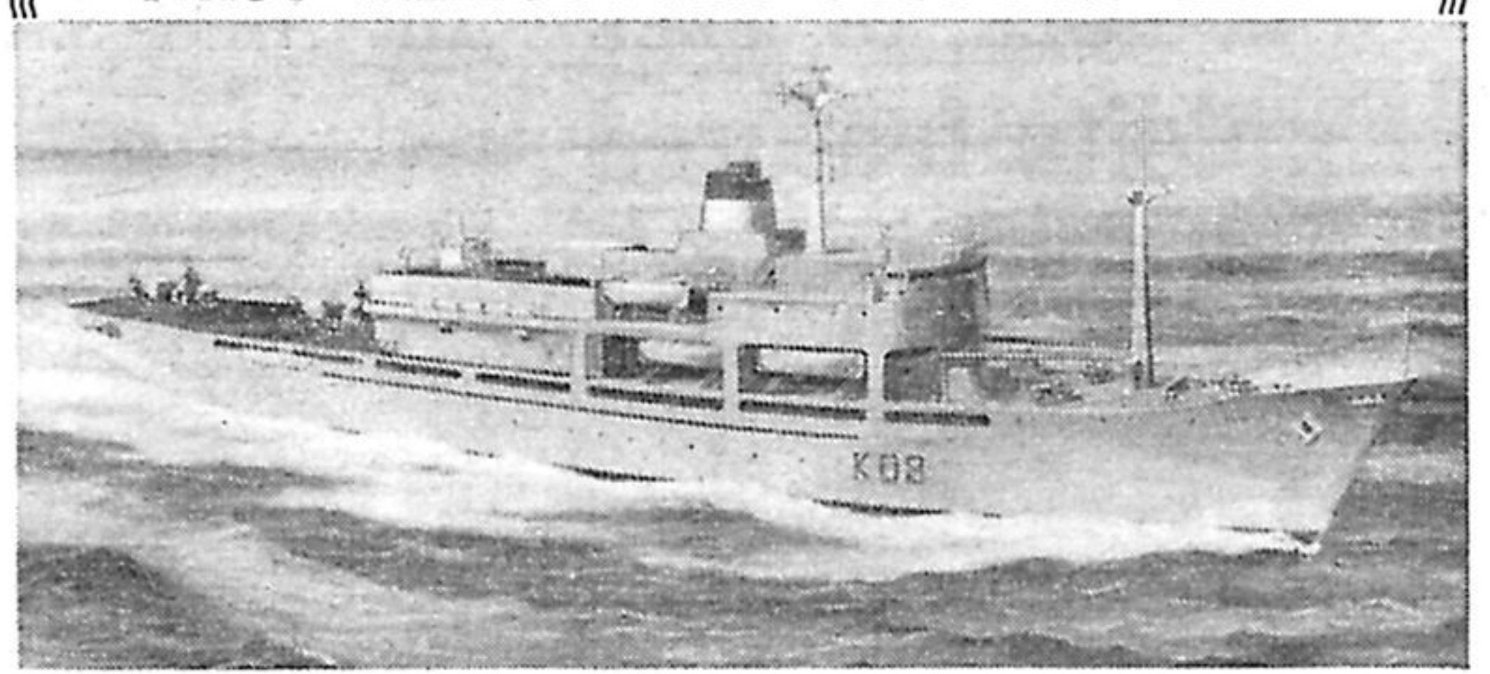
An artist's impression of the Royal Fleet Auxiliary Engadine, launched on September 15 at the yard of Henry Robb Limited, Leith. Named after a First World War seaplane carrier, Engadine is the Navy's first helicopter support ship. With a displacement of about 8,000 tons, the ship has been specially designed to meet naval training requirements in the flying, handling, and maintenance of helicopters.
