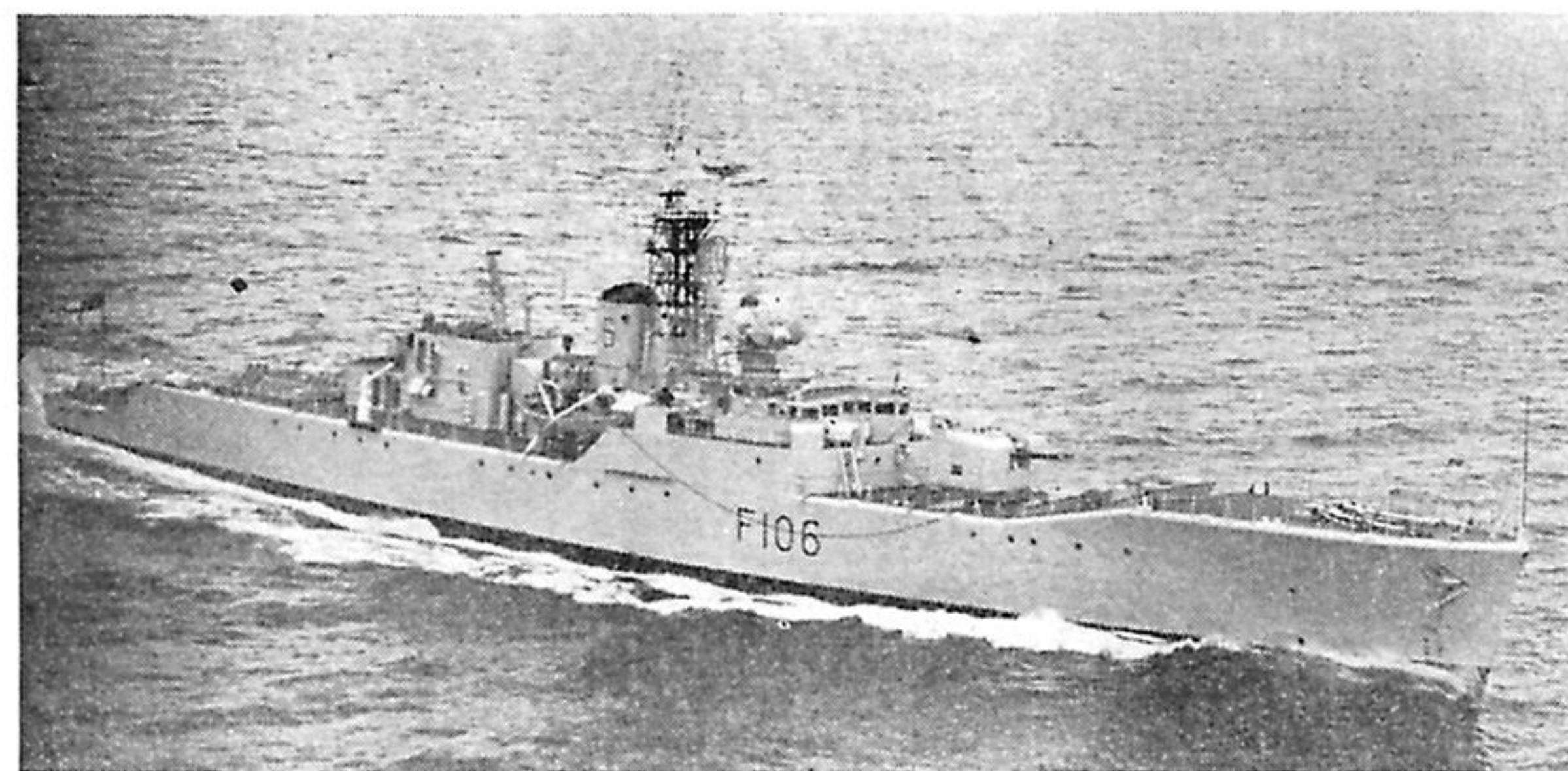
H.M.S. Brighton is a "Rothesay" class anti-submarine frigate built by Messrs. Yarrow and Co., Ltd., Scotstoun, 1959-1961. Capable of firing the Seacat guided missile, the "Rothesays" are basically similar to the "Whitbys" but with modifications in layout. All the ships of the "Whitby" and "Rothesay" class are named after seaside resorts and coastal towns
