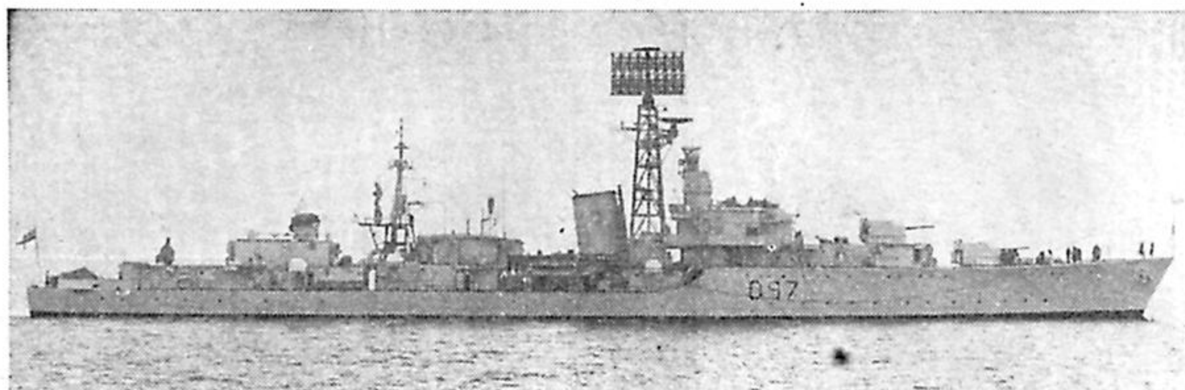
A destroyer open to visitors at Portsmouth during the August Navy Days this year is H.M.S. Corunna. Built as a "Battle" class destroyer by Swan, Hunter & Wigham Richardson Ltd., at Wallsend, Corunna has been converted into a Fleet Radar Picket (aircraft direction destroyer). The "double bedstead" radar aerial is a prominent feature. The complement of this ship, in peace, is 232 to 268. Displacement is 3,430 tons (full load)
