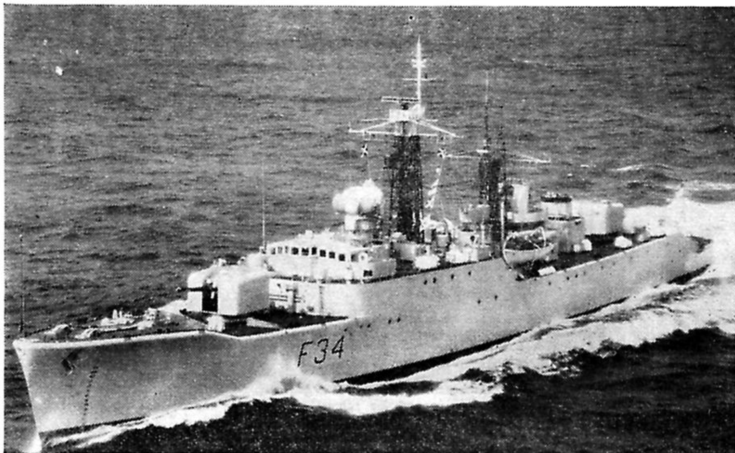
H.M.S. Puma, the anti-aircraft frigate designed primarily for the protection of convoys against aircraft
