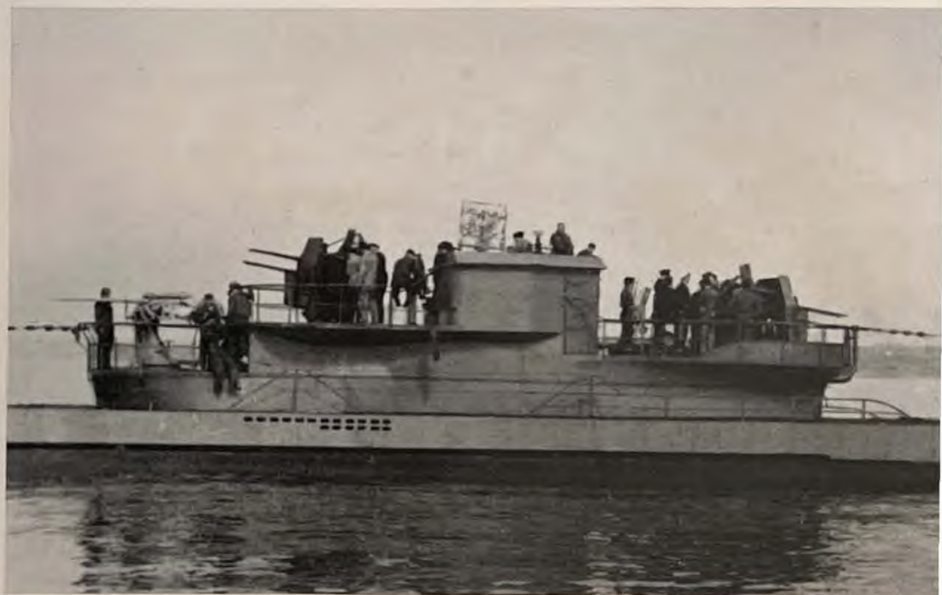
U.441 (A Type VII C, 770-ton Atlantic boat) fitted with special A.A. armament, armoured conning tower, and radar search receiver for work in the Bay of Biscay.
