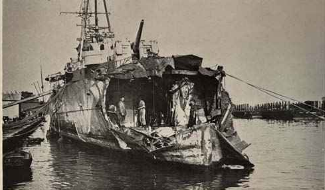
The damage caused to H.M.S. Delhi by a bomb hit, Algiers Bay, 20th November 1942.
