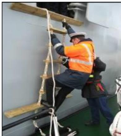
When boarding using a pilot hoist, a ladder must be rigged adjacent to the hoist and available for immediate use in the event of mechanical failure. The Pilot should climb the flexible short pilot ladder into the rigid upper section before indicating that he is ready to be hoisted at which point the pilot vessel should move away from the ship. The Pilot must ensure that no part of his clothing or equipment becomes entangled in the hoist mechanism.
